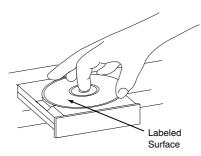
To close the drawer, press the appropriate Open/Close button 7 14 3 0 or gently press on the outside of the front cover of the disc tray. When the drawer is closed the word CLOSE will appear momentarily in the Information Display K, and the letters TOC will begin to flash in the display once the drawer s completely closed.
